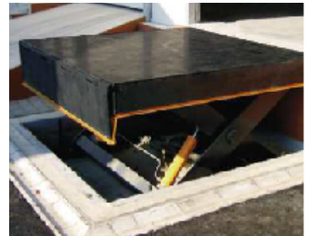
Lifting table with loading dock function
