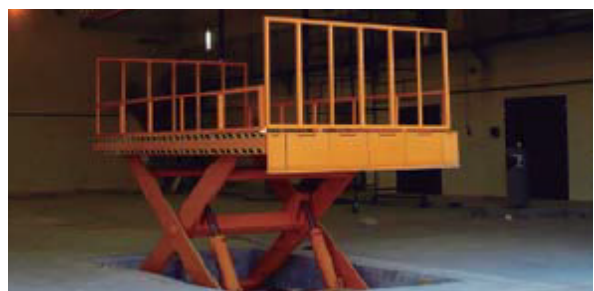
Single scissor lift with segmented lips and railings
