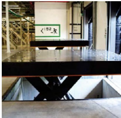
Lift table with studded platform
