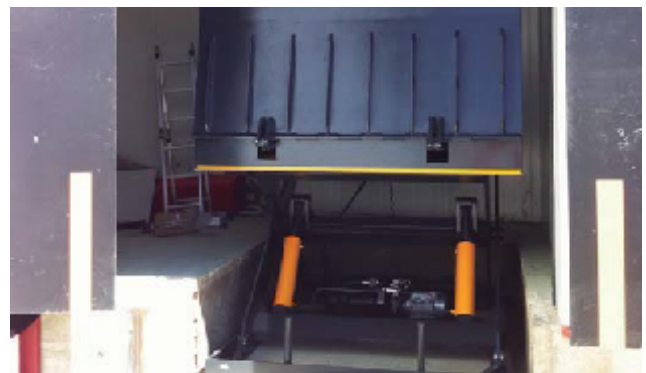
Single scissor lift with segmented lips and railings
